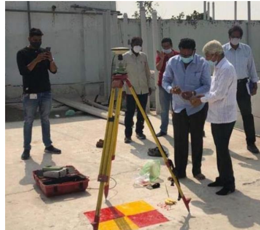
Figure 4-2: DGPS kept at MRP location in Solapur
